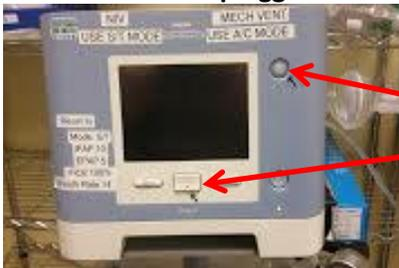
Press these two buttons for 3 seconds to activate the 'Setup' mode
