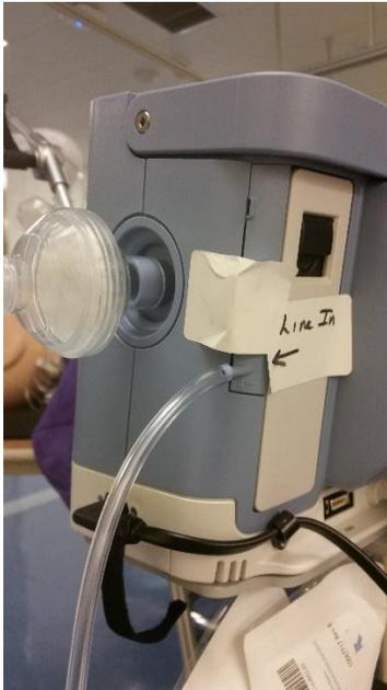
4. Press the 'alarm' and 'down' button – marked with BLACK arrows, for 3 seconds. This will allow 'Setup'. Machine must be plugged into the wall outlet, as Setup does not work off the battery (safety feature)
